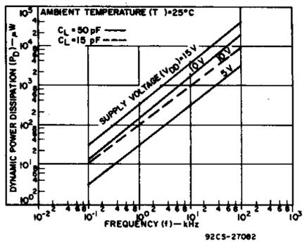
Fig. 7 - Typical dynamic power dissipation characteristics.
