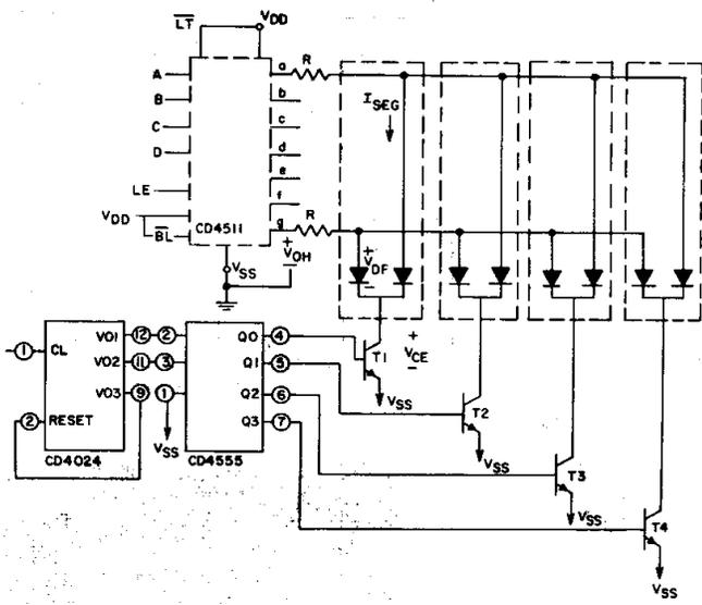
Multiplexing Scheme Showing 2 of 7 Segments Connected 92CM-27087RI
